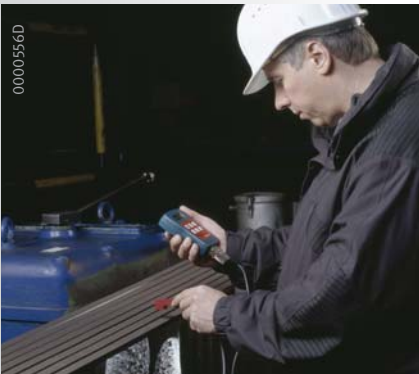
Corrective maintenance - Alignment with the TRUMMY2
