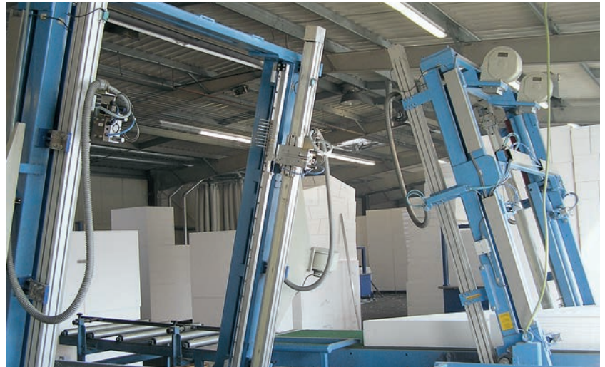
The cutting frame comprises two Schaeffler MKUVE20-B-ZR linear actuators, each equipped with a gripper system and nine single-wire feed units.
